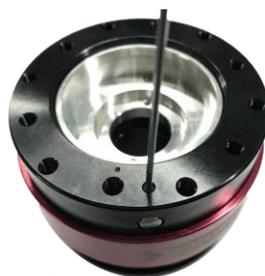
Use a wrench to loosen the screw
