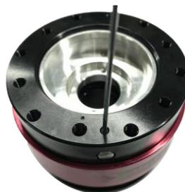
Use a wrench to loosen the screw
